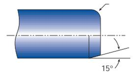
When using the centered arrangement, a small radius and adequate groove width should be used to ensure that the Tolerance Ring may be properly seated on the cylindrical surface.
